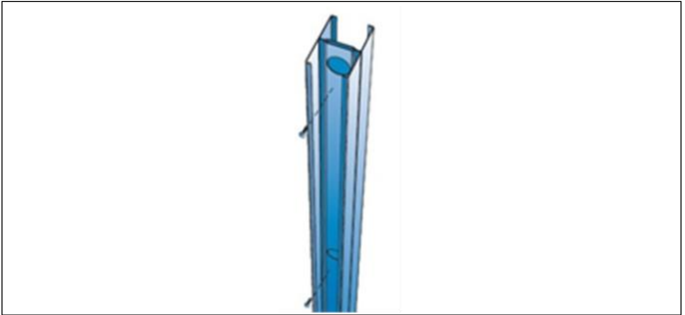
Figure 7 – Solidarisation des montants doubles
